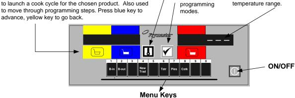
Press a menu key immediately after pressing a lane key to launch a cook cycle for the desired product. The keys are also used to enter names of products. Each button, when repeatedly pressed, accesses multiple letters or symbols. See example below.
